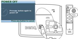
To protect the lamp, the projector will not respond to any commands during the cooling process.
