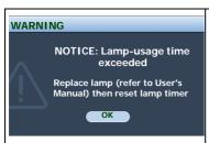
If this warning message displays, the projector will shut down in 40 seconds. The lamp MUST be replaced before the projector will operate normally.
