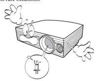
11. The lamp becomes extremely hot during operation. Allow the projector to cool for approximately 45 minutes prior to removing the lamp assembly for replacement.
