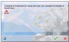
When decreasing the tension values to less than 1 a warning message appears. After confirmation, the minimum tension of 0.5 can be set.
