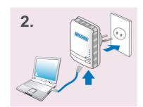
Create a secure network by a simply push off the network sync button.
