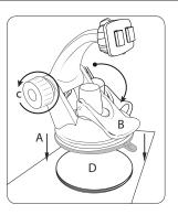
Step 6. Push the pedestal suction cup (A) down onto the disk (D). Flip the lever (B) down to secure the suction cup. Adjust the angle of the arm by loosening the adjustment knob (C).
