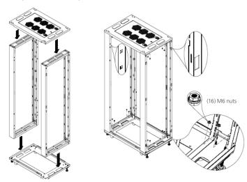
**STEP 2:** As shown in the diagram below, align the tabs of the horizontal supports to the slots in the vertical frame members and drop into place. Install the (2) bottom horizontal supports first. They are larger than the top/middle horizontal supports and must be installed in the bottom positions to allow the vertical rails to be installed. Use the blue and yellow plastic clips to attach the horizontal rails to the vertical frame.
