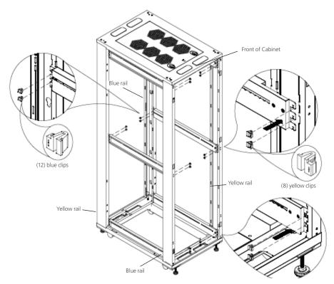
NOTE: Use the blue clips on the "blue rails" and the yellow clips on the "yellow rails." When you look directly at the front and rear of the cabinet (as shown in the diagram above), the left rail would use blue clips and the right rail would use yellow clips.
