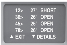
Figure C-4. Bad cable: far-end short
