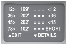
Figure C-7. Bad cable: wire map of shorted pair.
