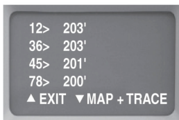
Figure 6-38. UTP pairs and length are displayed. Select MAP + TRACE for wiremap and tones.
