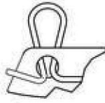
Figure 4-5. Create a loop from the power cable and feed it through the hole at the top front of the divider.
