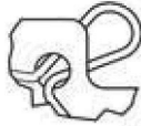
Figure 4-2. Loop the electrical cord and push it through the circular hole at the top rear of the divider.
