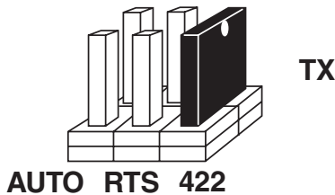
Figure 4-5. This jumper is in the “422” position. Note that the modem control outputs are only valid when Header E5 is in the 422 mode.
