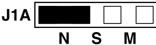
Figure 3-3. Header J1A, Normal IRQ Mode.
