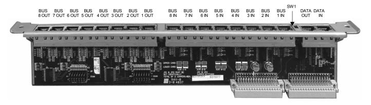
The 8-Port Expansion Card for the 8-User and 16-User ServSwitch Affinity models have two jumpers labeled JP1 and JP2 that control the numbering of an Affinity chassis' user ports. If the card is going into an 8-user Affinity chassis, follow the directions printed on the card's circuit board for the "lower" card, even though there is only one card and its slot is at the top of the chassis:
