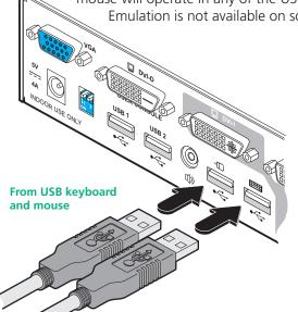
Note: The unit's True Emulation feature will read the full characteristics of the keyboard and mouse and will present those to each connected computer concurrently. This ensures that specialist keyboards and mice are fully supported.
