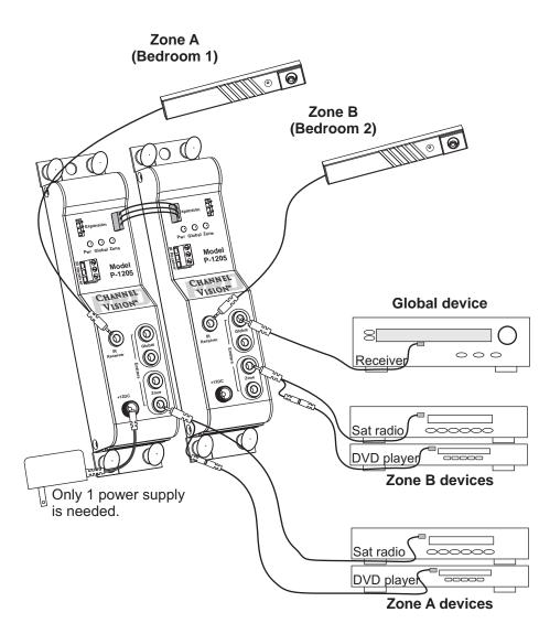
The diagram shown above, will create 2 IR zones that will allow for independent control of identical devices from the same manufacturer. The zone IR emitters will only respond to signals from the IR receiver that is in the same zone. The global IR emitters will respond to signals from any IR receiver in the system.
