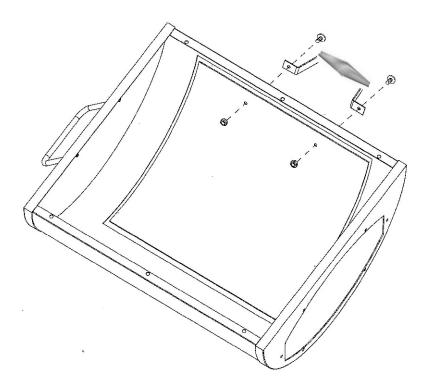
Attach firebox lid stop (item #24) using one M5 x 12mm Phillips head bolt and M5 hex nut.
