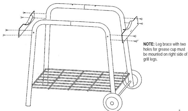
Install firebox support bracket (item #8) onto the holes on the left legs using two M6 x 15mm Phillips head bolts. **Do not tighten bolts until Step 6 is completed.**
