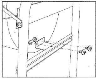
16 Install smokestack bracket (item #18) into grill lid (item #17 using two M6 x 15mm Phillips head bolts and M6 hex nuts.
