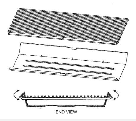
22 Use charcoal grate adjusters (item #14) to lower charcoal grate assembly into grill base (item #9). Rest charcoal grate adjusters on supports in grill base (item #9).
