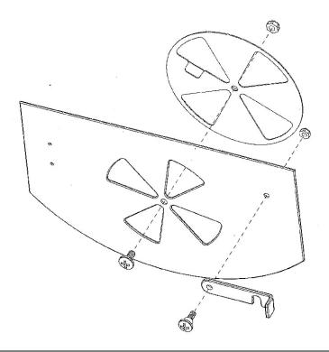
Connect firebox door hinge (item #29) to the outside of the door (item #30) and firebox base (item #34) using four M5 x 12mm Phillips head bolts and M5 hex nuts.
