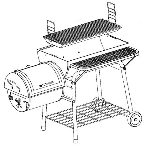
Install the warming rack (item #16) inside the grill lid (item #17). Insert the cotter pins through the holes from the outside of grill lid (item #17).
