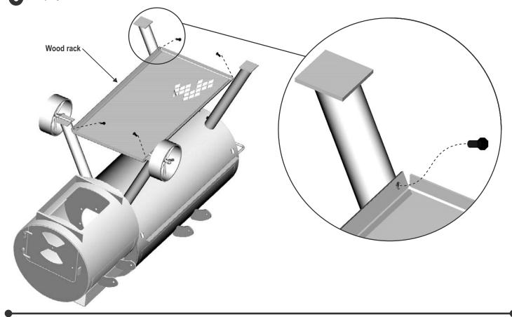
**MAKE SURE THAT LEG BOLTS ARE TIGHT ENOUGH SO THAT LEGS WON'T SLIP OFF OF POSTS.** Using three people, roll the unit over the handle brackets and stand it up onto its legs. Once standing, fully tighten the four leg bolts.
