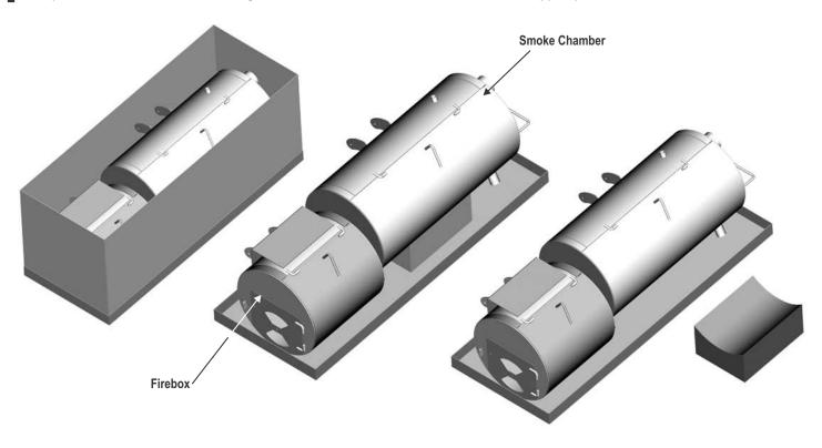
With one person on smoke chamber end, one person on firebox end, and one person holding both doors closed, roll the unit onto cardboard that was placed on the ground next to the unit. Unit should now be resting on its smoke chamber handle brackets with the leg posts pointing upward.
