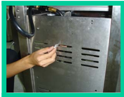
1a. Insert “threaded end” mounting bolt through top middle vent
