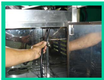
1a. Insert “threaded end” mounting bolt through top middle vent
