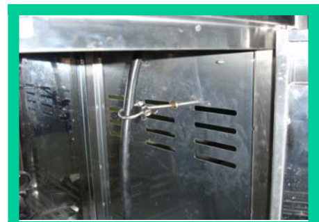
1b. Tighten nut with washer from the out side of panel with the included wrench
