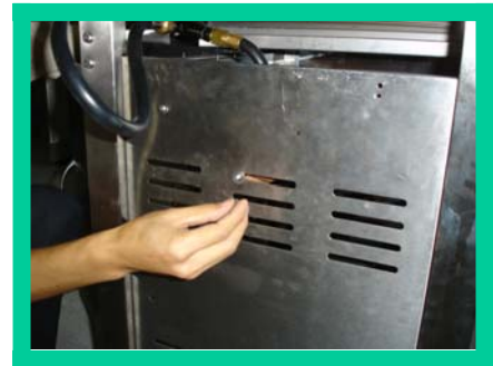
1b. Tighten nut with washer from the out side of panel with the included wrench
