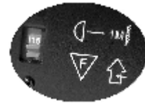
Figure 1 - AC Voltage Switch
