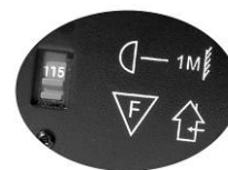
Figure 1 - AC Voltage Switch
