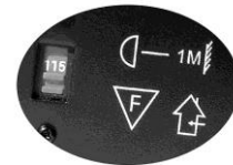
AC Voltage Switch
