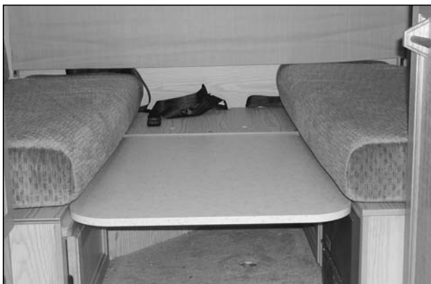
Picture B-P13: Placement of support pieces for the double bed, (Versatile model).
