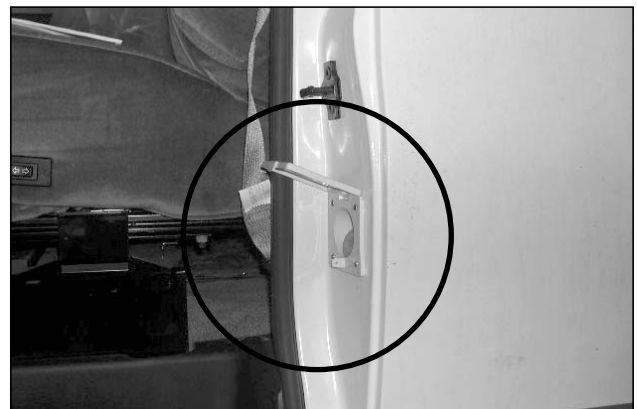
Picture G-P2 : The gravity fill, (front driver door post, on all models).
