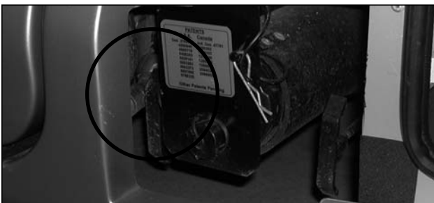
Picture G-P23: Exterior fresh water drain valve, (170 model).
