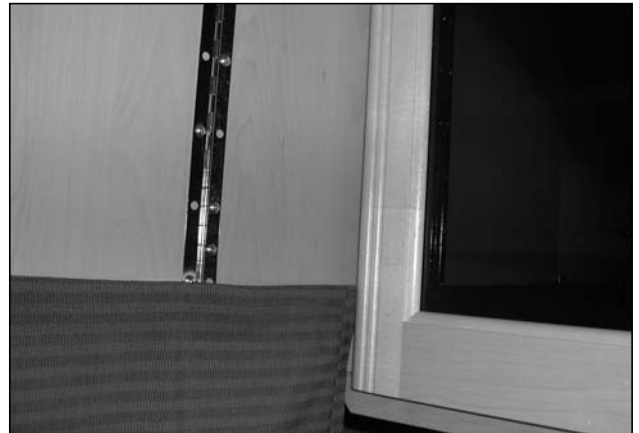
Picture B-P27: Position of rear privacy door when secured behind A/V door, (190 Popular model).
