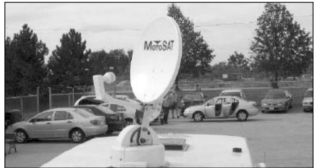
Picture B-P48: Satellite in "up" or ready for use position.
