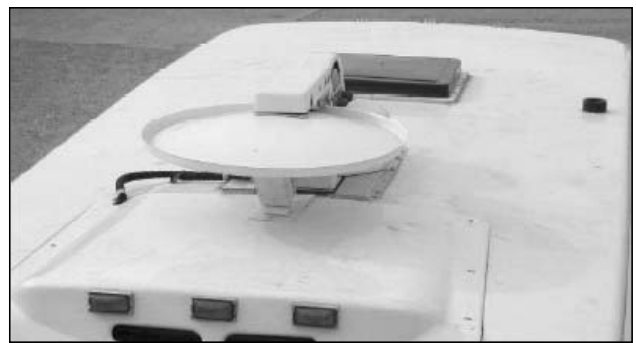
Picture B-P49: Satellite in "stowed" or travel position.
