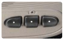
This programmable transmitter can store three frequencies for items such as a garage door opener, entry door lock or security system.
