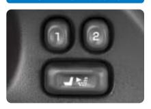
The memory seat controls are located on the driver door. They program and recall driver seat position and outside mirror settings for up to two drivers.
