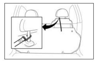
8. Clip the hook to the front seat head restraint to keep the rear seat secure.
