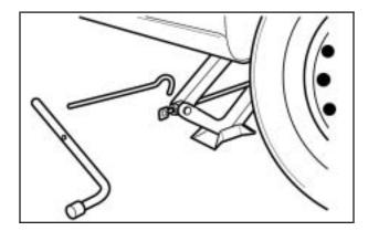
8. Insert the jack handle into the jack and the wheel wrench onto the end of the jack handle.
