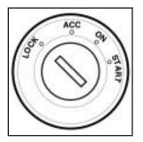
The ignition switch has four different positions.
