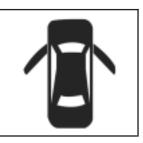
The door ajar light comes on and stays on until all doors, trunk and liftgate are closed and completely latched.
