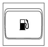
To open the fuel filler door, pull up on the release lever with this symbol on it. It is located on the floor on the outboard side of the driver seat.
