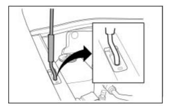
Before closing the hood, be sure all the filler caps are on properly. Then lift the hood to relieve pressure on the hood prop. Remove the hood prop from the slot in the inner fender and return the prop to its retainer. Lower the hood 12 inches (30 cm) above the vehicle and release it so it fully latches. Check to make sure the hood is closed and repeat the process if necessary.
