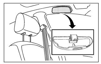
For vehicles with this feature, the sunglasses storage compartment is located above the driver's door. To open, pull down and hold the upper part of the cover. Release the cover and the compartment will automatically close.
