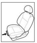
Pull up and hold the bar located under the front of the seat to unlock it.
