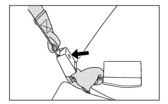
3. Detach the center safety belt from the mini buckle by inserting the key into the slot in the mini buckle, pressing the release button, and allowing it to retract.
