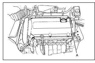
2. Remove the extension cord from the trunk. Open the hood and connect the electrical cord (A) with the extension cord. 3. Plug the extension cord into a normal, grounded 110-volt AC outlet.
