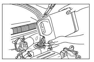
3. Fill the coolant surge tank with the proper mixture to the Maximum mark on the coolant surge tank. Wait about five minutes, then check to see if the level is below the mark. If the level is below the Maximum mark, add additional coolant to bring the level up to the mark.
