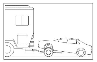
The vehicle can be towed from the front using a dolly. To tow the vehicle using a dolly, follow these steps:
