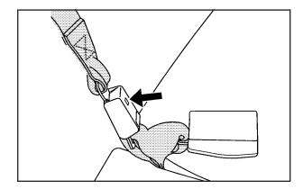
4. Detach the center safety belt from the mini buckle by inserting the ignition key into the slot in the mini buckle, pressing the release button, and allowing the belt to retract.
