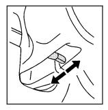
The tilt wheel lever is located underneath the steering column slightly to the left.
