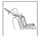
If the position you are using has an adjustable headrest or head restraint and you are using a single tether, route the tether under the headrest or head restraint and in between the headrest or head restraint posts.
