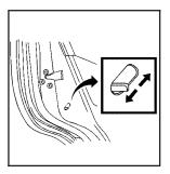
Your vehicle has rear door security locks on each rear door that prevent passengers from opening the rear doors from the inside.
