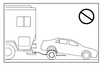
*Notice:* Towing the vehicle from the rear with the front wheels on the ground could cause transmission damage. Do not tow the vehicle from the rear with the front wheels on the ground.
