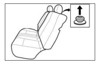
4. Pull up the release knob, located on the top of the seatbacks, and fold the seatbacks forward and down.
