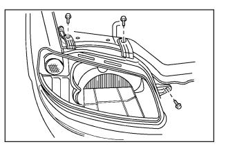
10. Reinstall the headlamp assembly using the three bolts.
