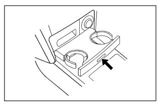
Two cupholders are located in the center instrument panel, below the climate control system. To use the cupholder, push in on the cover, then pull it out. After use, push in the cupholder until it latches.
