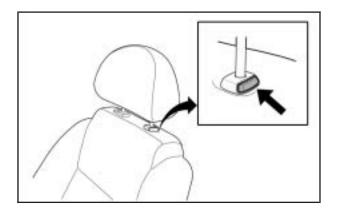
Pull the head restraint up to raise it. To lower the head restraint, press the button, located on the top of the seatback, and push the restraint down.
