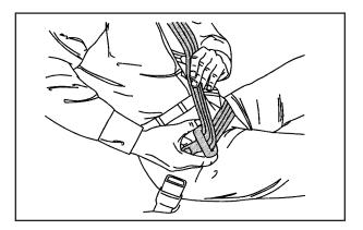
3. If the belt stops before it reaches the buckle, tilt the latch plate and keep pulling until it can be buckled.
