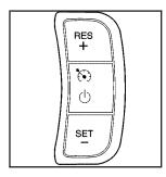
The cruise control buttons are located on the right side of the steering wheel.
