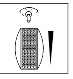
The thumbwheel for this feature is located on the instrument panel to the left of the steering column. Turn the thumbwheel to brighten or dim the lights.
