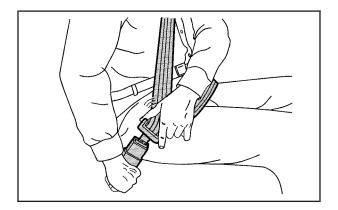
Push the latch plate into the buckle until it clicks. If the latch plate will not go fully into the buckle, check if the correct buckle is being used.
