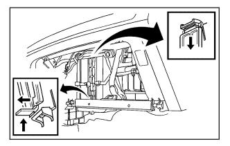
3. Remove the filter cover by pressing in on the bottom retaining tab and pulling the cover down.
