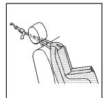
If the position you are using has a headrest or head restraint and you are using a dual tether, route the tether under the headrest or head restraint and in between the headrest or head restraint posts.
