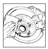
12. Remove any rust or dirt from the wheel bolts, mounting surfaces and spare wheel. 13. Place the compact spare tire on the wheel-mounting surface.
