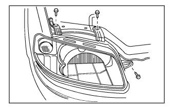
10. Reinstall the headlamp assembly using the three bolts.
