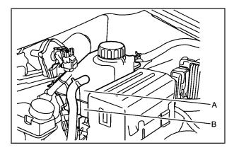
The engine coolant surge tank is located in the rear of the engine compartment on the driver side of the vehicle. See *Engine Compartment Overview on page 5-14* for more information on location.
