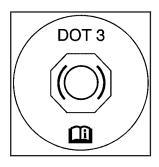
The vehicle has one reservoir for both the brake and clutch hydraulic systems. It is filled with DOT-3 brake fluid.
