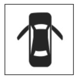
If one of the doors, trunk or liftgate is not closed properly while the ignition is on, the door ajar light on the instrument panel comes on and stays on until the doors are closed.
