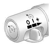
The cruise controls are located at the end of the multifunction lever.
