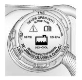
The engine coolant surge tank is located toward the rear of the engine compartment on the driver side of the vehicle. See *Engine Compartment Overview on page 10-10* for more information on location.
