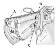
When you have the transmitter with you, you may also unlock and open the door by squeezing the door handle sensor (A). You do not have to press the unlock button on the transmitter. You will be able to open the door when you press the door handle sensor and the vehicle recognizes your keyless access transmitter. When the passenger door is opened first, the driver's door will also unlock.
