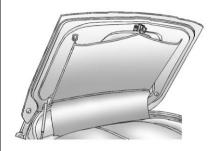
Grasp the loop at the rear center of the shade and wrap it around the striker assembly.
