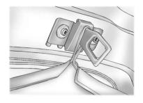
4. Push the loop to the top of the striker (base plate).
