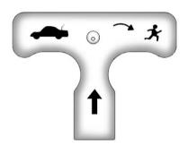
Notice: Do not use the emergency trunk release handle as a tie-down or anchor point
