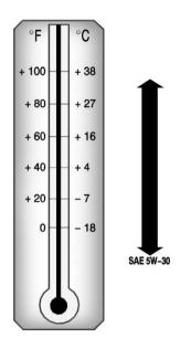
Cold Temperature Operation: In an area of extreme cold, where the temperature falls below −29°C (−20°F), an SAE 0W-30 oil should be used. An oil of this viscosity grade will provide easier cold starting for the engine at extremely low temperatures. When selecting an oil of the appropriate viscosity grade, be sure to always select an oil that meets the required specification, dexos™. See "Specification" for more information.
