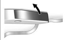
Pull the door release handle located on the floor next to the seat.
