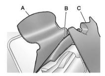
Lift the rear edge (B) of the convertible top to its full-up position by first raising the front edge (A).
