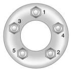
Tighten the wheel lug nuts firmly in a crisscross sequence as shown.
