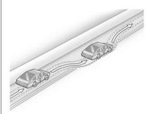
If the level of the shoulder is only slightly below the pavement, recovery should be fairly easy. Ease off the accelerator and then, if there is nothing in the way, steer so that the vehicle straddles the edge of the pavement.
