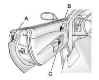
When you have the transmitter with you, you may also unlock and open the door by squeezing the door handle sensor (A).
