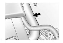
4. With the coolant surge tank pressure cap off, start the engine and let it run until the upper radiator hose can be felt getting hot. Any time during this procedure, watch out for the engine cooling fan.
