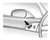
On vehicles with the memory feature, the controls on the driver door are used to program and recall memory settings for the driver seat, outside mirrors, and the telescopic steering column.
