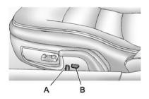
On vehicles with power lumbar and side bolsters, the controls are located on the outboard side of the seat.
