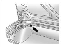
Pull the divider up and snap it onto the snaps on both sides of the trunk.
