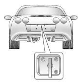
Press the hatch/trunk release button located on the rear of the hatch/trunk lid above the license plate, as long as you have your transmitter with you.
