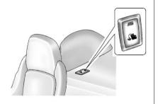
The top tether anchor is located under the cover behind the passenger seat.
