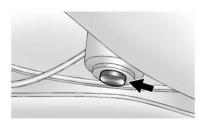
7. Tilt the driver's seatback forward and press the tonneau cover release button located on the underside of the tonneau cover (C) behind the driver's seat. Then raise the tonneau cover (C). If the tonneau cover does not release and three chimes are heard, check to make sure the trunk lid is closed. Also, the cover will not release if the vehicle alarm is armed.
