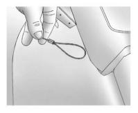
Open the tonneau cover by pulling the emergency release cable.
