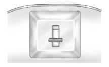
To fold a seatback forward, lift the latch on top of the backside of the seat. The seatback locks when folded down.
