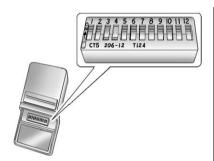
To verify that the garage door opener is a Fixed Code unit, remove the battery cover on the hand held transmitter supplied by the manufacturer of the garage door opener motor. If there are a row of dip switches similar to the graphic above, the garage door opener is a Fixed Code unit. If you do not see a row of dip switches, return to the previous section for Programming Universal Home Remote – Rolling Code.
