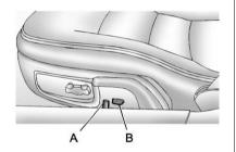
On vehicles with power lumbar and side bolsters, the controls are on the outboard side of the seat.
