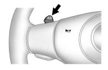
To operate the Manual Paddle Shift system, the automatic transmission shifter must be in S (Sport Mode). The system is activated by pushing the paddle, above the steering
