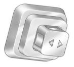
For vehicles with this feature, the telescopic steering column switch is located on the right side of the steering column.
