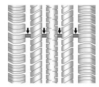
One way to tell when it is time for new tires is to check the treadwear indicators, which appear when the tires have only 1.6 mm (1/16 in) or less of tread remaining. See *Tire Inspection on page 10-72* and *Tire Rotation on page 10-72* for additional information.
