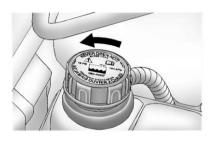
When the cooling system, including the coolant surge tank pressure cap and upper radiator hose, is no longer hot, remove the pressure cap.
