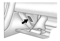
If moving the transmitter to different locations within the vehicle does not help, place the transmitter in the glove box transmitter pocket with the buttons facing to the right and then press the START button.
