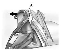
Pull the convertible top up by firmly gripping the front edge (A) near the center and applying a brisk upward and forward motion to get the top in the full-up position.
