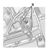
Lift the vehicle with the jack, making sure the jack spans at least two of the crossmember ribs (B).
