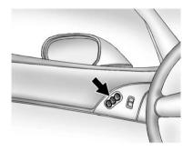
On vehicles with the memory feature, the controls on the driver door are used to program and recall memory settings for the driver seat, outside mirrors, and the telescopic steering column, if equipped.
