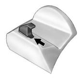
Insert the roof panel so that the outside front edges line up between the receiver covers.
