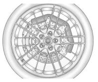
A rotor protector should always be installed before any wheel removal. The protector can be installed by feeding it through the wheel spokes and slipping it over the outer edge of the rotor. Leave the protector in place, over the rotor edge, until the wheel is re-installed. Rotor protectors are available through your dealer.
