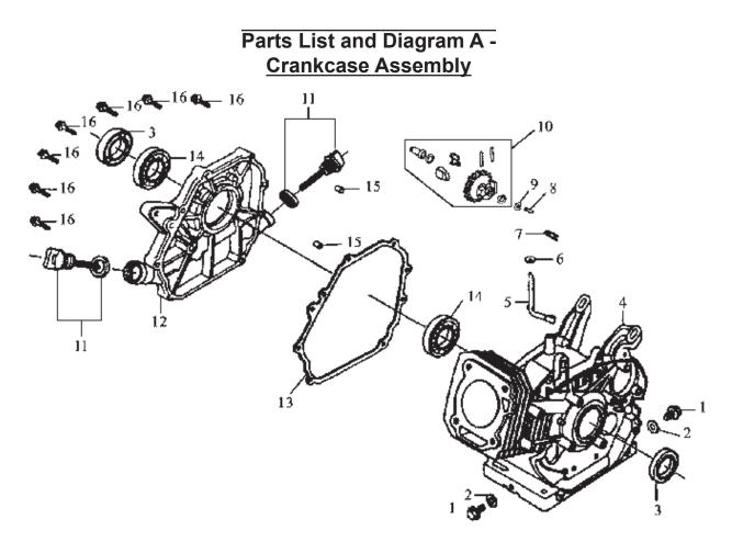
**NOTE:** All part numbers listed on the following pages have a letter suffix. For example, the Crankcase Cover shown in the above diagram is part # 12a. Whenever referring to engine sub-assembly parts, be sure to include the complete part number including the letter suffix.
