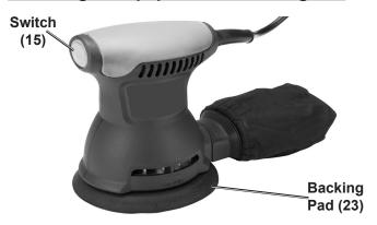
The Sanding Disc is attached by Hook and Loop to the Backing Pad. Place the Sanding Disc on the Backing Pad lining up the 8 holes so that the dust can be collected into the Dust Bag.
