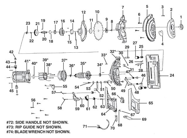
\*NOTE: PARTS #32\* THROUGH 41\* MAY NOT BE ORDERED INDIVIDUALLY, BUT MUST BE ORDERED AS A COMPLETE MOTOR ASSEMBLY (PART #76\*).
