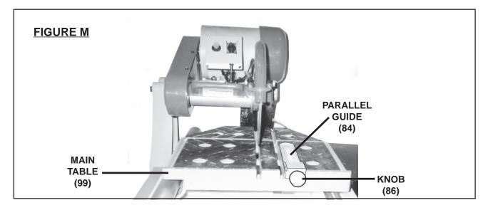
3. Attach the Angle Block (85) as you did the Parallel Guide, using the two Knobs (86) on the side of the Guide. Use the cutting groove in the middle of the Main Table to brace the edge of the tile as the tile is slid underneath the Saw Blade (65). (See Figure N.)
