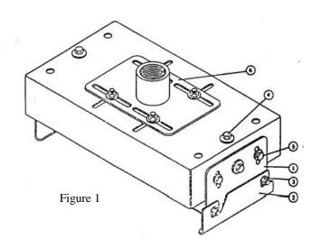
5. Tighten securely using the 5/16-18 flange nuts (3).
