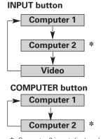
Computer 2 is not displayed when the COMPUTER IN 2/COMPONENT IN/MONITOR OUT terminal is used as Monitor out.
