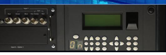
Direct key access to the most-used major functions and auto set-up of sources with correct brightness, contrast and position means operation and set-up of the Christie Mirage Series are intuitive.
