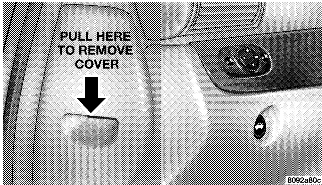
Fuse Panel Cover
