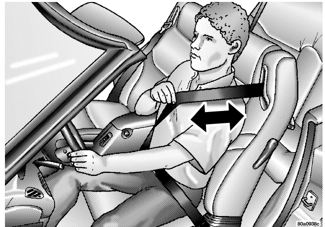
Removing Slack From Belt
