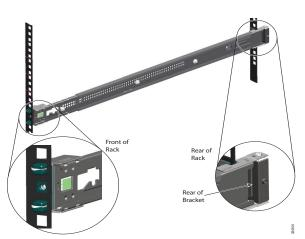
Secure the other outer slide rail to the rack by repeating the previous steps.
