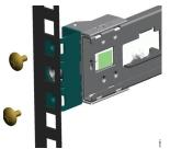
Align the slide rail to the rear rack post. Secure it with two of the included Phillips pan-head screws (F).
