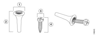
1 8 mm/0.32 in 2 25 mm/0.98 in 3 6.5 mm/0.26 in 4 18.6 mm/0.73 in
