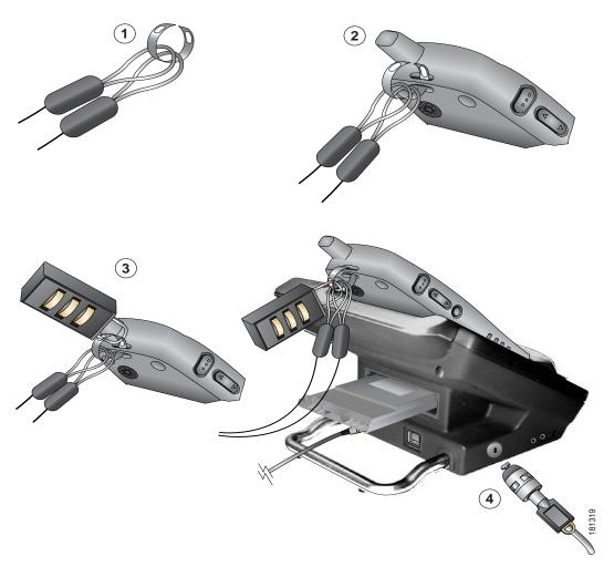
You can secure your Cisco Unified Wireless IP Phone 7921G Desktop Charger by using a laptop cable lock. The lock connects to the security slot on the side of the desktop charger, and the cable can be secured to a desktop. The diagram shows where to insert the lock.
