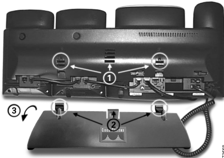
Figure 4-8 Part Connections on the Footstand and Support Bar
