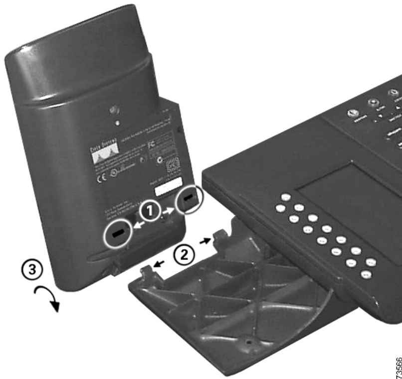
Figure 4-4 Part Connections on the Expansion Module and Support Bar
