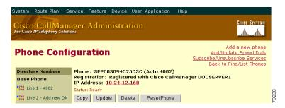
Step 7 Reset the phone after making changes to apply the new settings. See the "Resetting a Phone" section on page 45-8.
