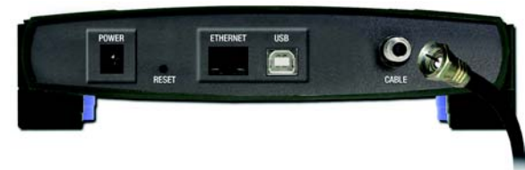
Figure 3-1: Connect the Coaxial Cable
