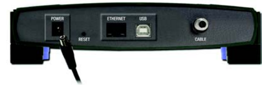
Figure 3-6: Connect the Power Cable
