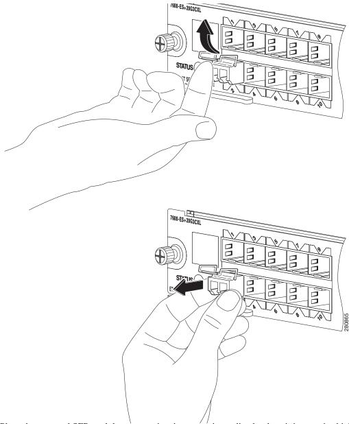
Figure 5-2 Removing a Bale Clasp SFP Module
