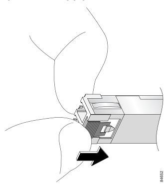
**Step 5** With the tab still pushed, carefully pull the SFP module from the port as shown in Figure 5-12.
