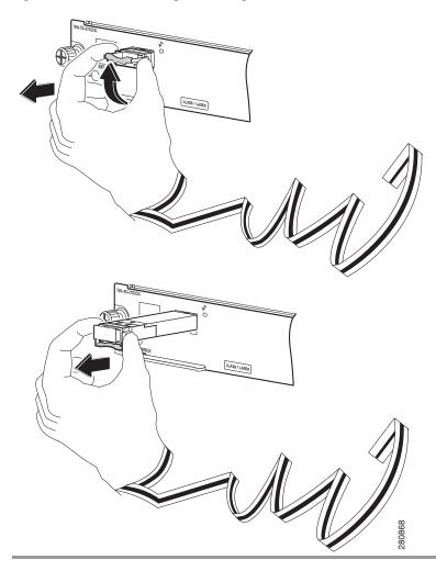
Removing and Installing XFP Modules
