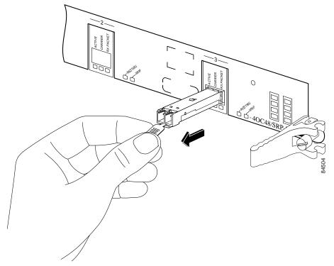
Step 4 Place the removed SFP module on an antistatic mat, or immediately place it in a static shielding bag if you plan to return it to the factory.
