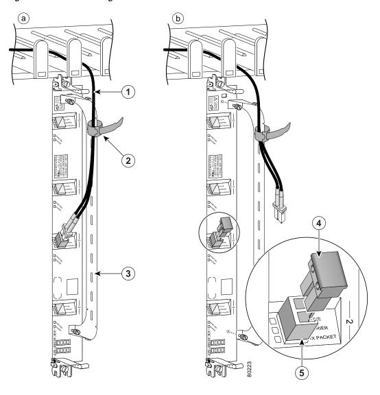
Figure 40 Disconnecting Line Card Interface Cables
