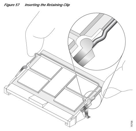
The clip is properly installed when the clip detente protrudes below the strain relief and plastic latch. (See Figure 58.)
