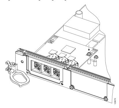
Step 6 Use a Phillips screwdriver to insert and tighten the two screws on the faceplate of the line card, 3 to 5 in-lbs, as shown in Figure 15.
