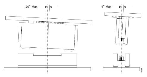
**Step 3** Ensure that the connector guide pins are aligned. Once the connector is engaged, apply gentle pressure with your thumbs to the two rear outer corners of the EPA, as shown in Figure 11 and Figure 12.
