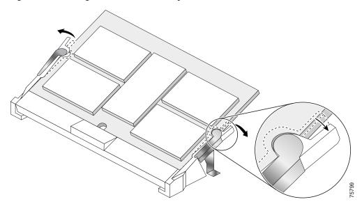
Step 6 As the SODIMM is released, it positions itself at a 45-degree angle. Gently pull the SODIMM module out of the socket. Continue to keep the module at a 45-degree angle until it is completely removed from the socket guides. (See Figure 53b.)
