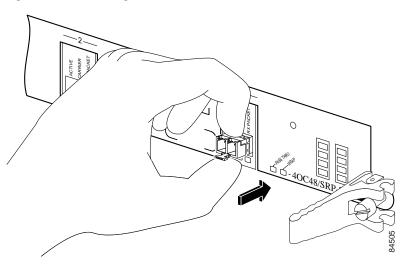
Figure 25 Installing an Actuator Button SFP Module
