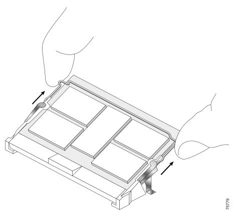
Figure 51 Remove Retaining Clip from Memory Module Socket
