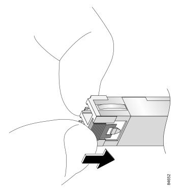
Step 5 With the tab still pushed, carefully pull the SFP module from the port as shown in Figure 28.
