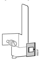
Figure 31 Multiport Line Card Cable-Management Bracket
