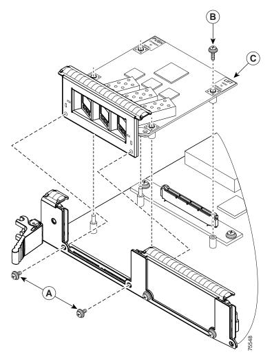
If the EPA bay is to remain empty, install an EPA blank (Product Number MAS-EPA-BLANK=) to keep dust out of the line card and to maintain proper airflow and EMI through the line card and chassis.
