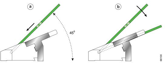
Step 9 Gently press the SODIMM down using your index fingers, distributing even pressure across the module until it locks into the tabs. (See Figure 56b.)
