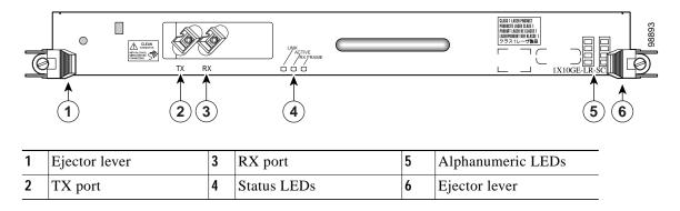
Table 7 summarizes the optics and connectors used by the 1-Port 10-Gigabit Ethernet line card.
