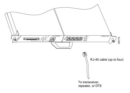
**Note** VIP configurations using only one 4E port adapter and a port adapter blank, or two 4E port adapters, are currently not supported. The FE-TX and 4E port adapters have a handle attached, but this handle is not shown to allow a full view of detail on each port adapter's faceplate.
