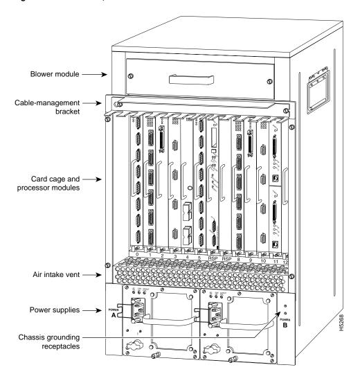
Figure 6 Cisco 7513, Interface Processor End
