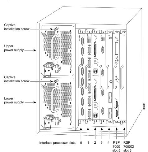
Figure 2 Cisco 7000, Interface Processor End
