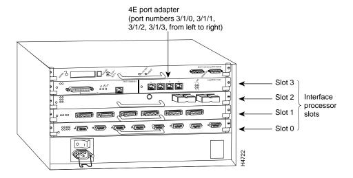
Figure 31 10BASE-T Interface Port Number Example (Cisco 7505 Shown)
