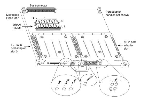
Figure 1 VIP with One FE-TX and One 4E Port Adapter (Product Number VIP-FE-TX/4E[=])
