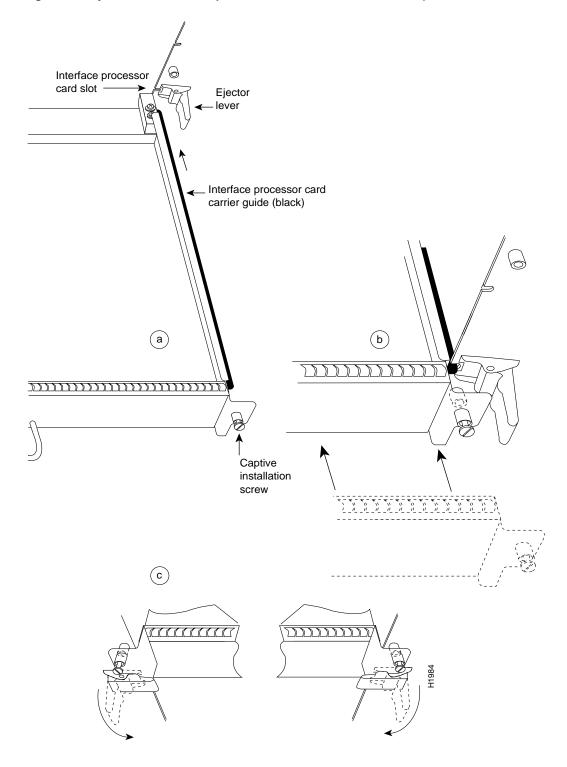
Figure 8 Ejector Levers and Captive Installation Screws on the VIP (Horizontal Orientation Shown)
