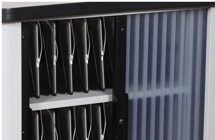
Figure 4-1. Sync cables in cart unplugged from iPads.
