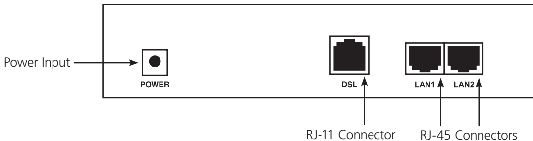
Figure 2-5. Rear panel, VDSL2 PoE Ethernet Extender (PD), Standard unit.
