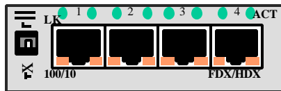
Figure 4.3 : Up-link push-button on RJ-45 4-port
