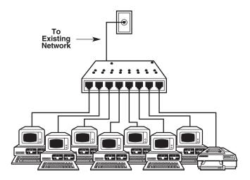
9-Port Personal MiniHubs may also be used standalone to network a local personal multi-user system, as shown below. Up to nine RJ-45 user ports are available where only 10BASE-T wiring is used, and full-length Ethernet segments are supported on all segments. In this application, set the Up-Link switch to the straight-through or "===" position, so that the MiniHub's rear port is a user port, not an up-link to another hub.
