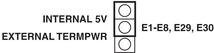
Figure 5-1. Internal terminator-power jumpers.
