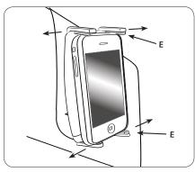
Step 1. If necessary, adjust the support legs (E) on top and bottom by sliding them laterally to avoid any buttons or ports that may be on your phone.
