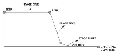
**Stage One** — Rapid Start Charge at 10 amps delivers maximum charging amperage to "wake up" any serviceable 12 volt battery and allows for quick engine starting in just 8 minutes (based on a midsize vehicle battery at 50% charge level). When battery reaches a maximum safe predetermined voltage, the charger will automatically signal a "beep" and move into Stage 2 of the charging process.
