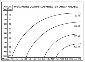
For example, as shown in the above graph, using a 400 A/h battery (batteries), if the average power usage will be 1000 watts, the operating time will be about 150 minutes. A larger capacity battery will deliver more operating time between recharges.
