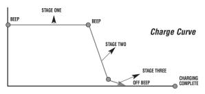
to allow for the maximum proper internal chemical energy transfer. At the end of Stage 2, the charger will automatically move into Stage 3 charge mode.
