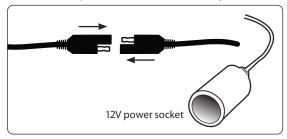
Step 2. Carefully reconnect vehicle battery cables. Insert a 12V accessory into the 12V socket to power your mobile device (not included, sold separately).
